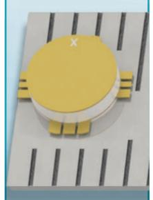
VIDA's 6 ~ 24 GHz patented Differential Oscillator Module features excellent phase noise and spurious response. The small size fits all magnetic packages. Use your existing magnetic tuning package or design your own with VIDA application notes. Standard Oscillator package is a sealed 1mm thick by 4mm diameter pill package.
