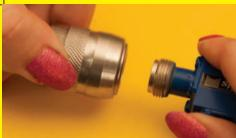
6. Keep fingers on "Back Nut" to ensure that "Lock Nut" cannot slide back and pull the connector off.
