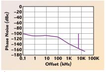
Fig. 3 Worst spur, fixed 50 MHz reference, output frequency = 2 GHz.
