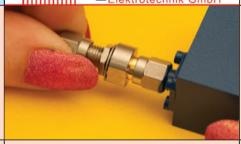
3. Just slide the Push-On SMA female Connector onto any standard SMA male. The connection is securely done in seconds.
