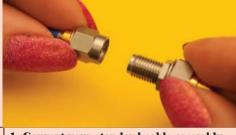
1. Convert your standard cable assembly into a Push-On Assembly by threading the standard female side of the adapter onto the male connector of the assembly.
