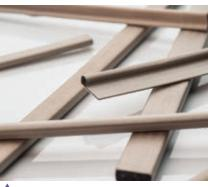
▲ Fig. 2 Metalized fabric gaskets are manufactured with a polyurethane foam core and nickel-plated copper-conductive fabric.
